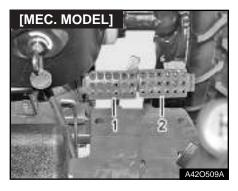
(1) Brake pedal (LH) (2) Brake pedal (RH)
