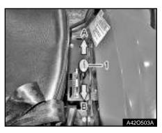
(1) Hitch control lever (A) Lowering (B) Lifting
