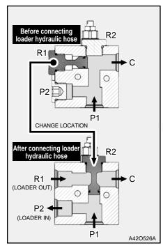
When installing a loader, the plug of the port R1 should be fit to the port R2 to enable correct operation of the loader.
