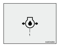
(1) Engine Oil Pressure Warning Lamp
