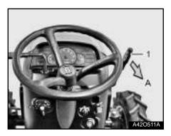
(1) Hand throttle lever (A) Engine rpm increases
