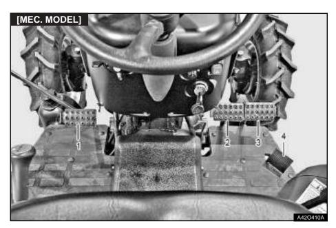
(1) Clutch Pedal (2) Left Brake Pedal
