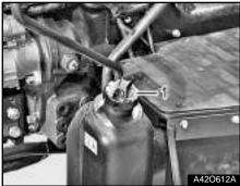
Turn the main switch to the "ON" position. If the fuel gauge needle is pointing the red area, open the fuel cap, and then fill the fuel tank full through the oil filler. Open the engine side cover and check if there is leakage.
