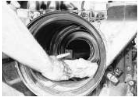
Fig3-13 Clean the Shell and Dust Cup
