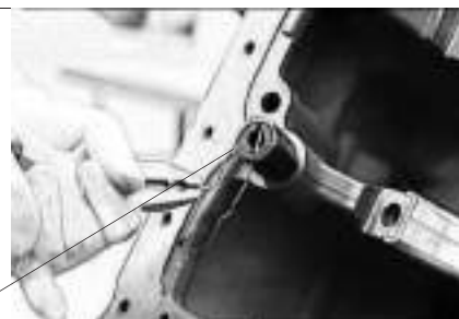
Fig 5-2 Pressure Limiting Valve of Oil Pump
