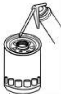
Fig3-11 Replace Diesel Fuel Filter Element
