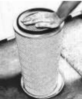
Fig3-14 Rubber Ring Installation
