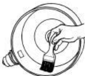
Fig 3-5 Clean Dust Accumulator
