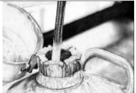
Fig 5-13 Freezing of Intake & Exhaust Valve Seats in Liquid Nitrogen
