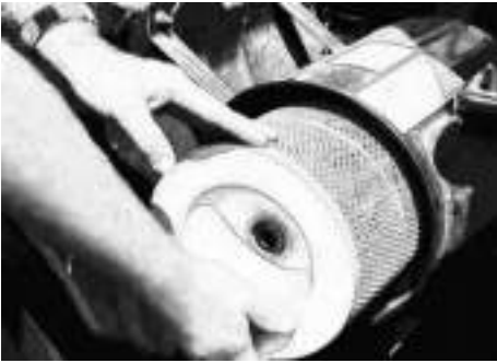
Fig3-13 Clean the Shell and Dust Cup
