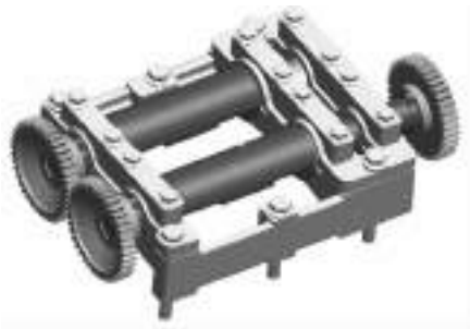
Fig 5-27 Double-shaft Balance Mechanism
