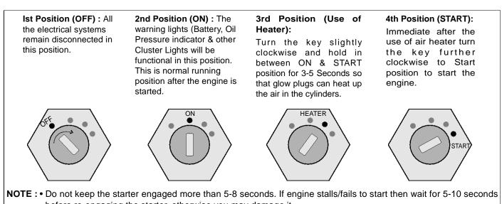
before re-engaging the starter, otherwise you may damage it.Keep the switch in OFF condition when engine is also in OFF condition.
