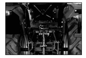
2. Apply a small quantity of oil to the depth control handle and mount it to the support. Fit a washer on the handle, mount it to the frame, fit another washer from the lower side, fasten with a castle nut so that the handle turns lightly and lock with a cotter pin. (Fig. 2)
