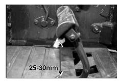
Note: Difference in the free play will lead to unbalanced brakes. the tractor can slew, in the event of violent braking, the wheel on which the brakes are applied locks and the tyre wears out quickly. During Road Operations Both the brake Pedals should be locked
