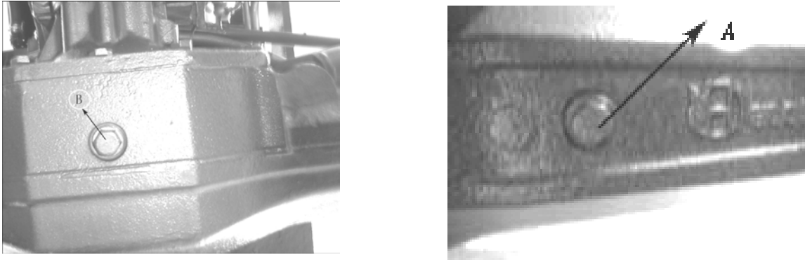
Fig. 5-4 Oil level inspection of the front drive housing
