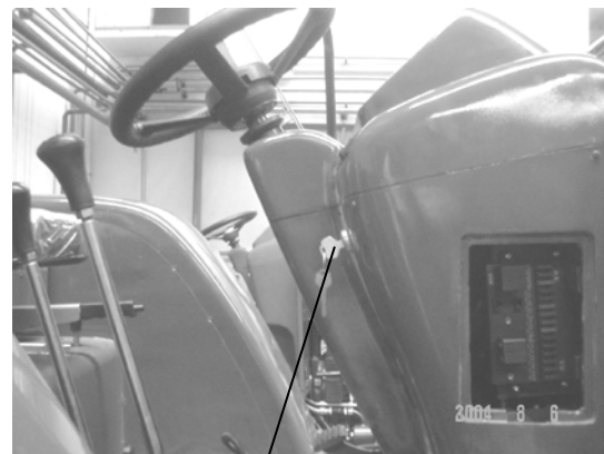
Fig 3-28 Battery starting 1. Ignition lock key
