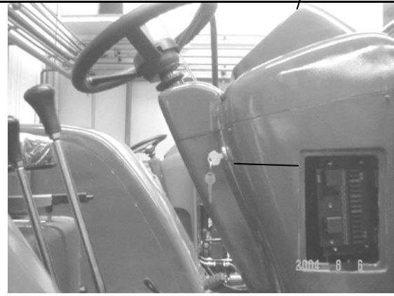
Fig. 3-78 Central electrical control box
