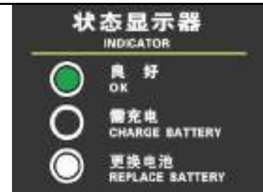
Fig 5-1 Inspection of battery condition
