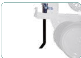
Ripper for direct seeding on light soil.
