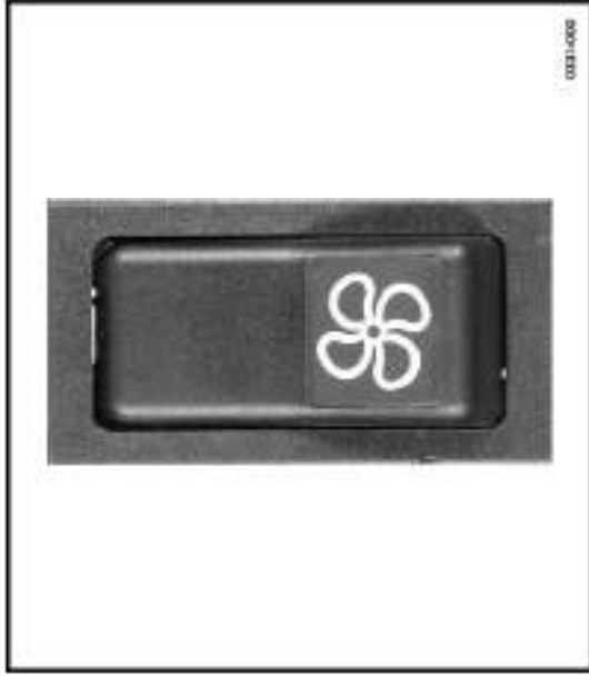
331 Toggle switch ventilation
