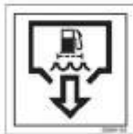
Water sump fuel filter outlet
