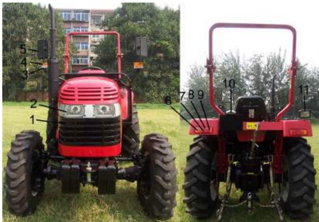
Fig.6-37 Distribution of lamplight and signal
