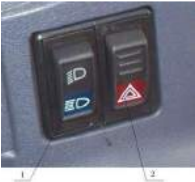
Figure 2-12 Right Rocker Switch Combination
