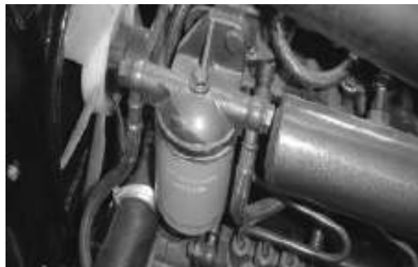
Figure 4-24 Fuel Filter Maintenance
