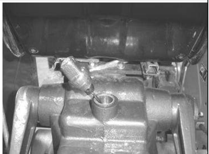
Figure 4-29 Lifter Oil Dipstick
