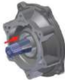
6 montare la bussola conica Fit the special conic bushing
